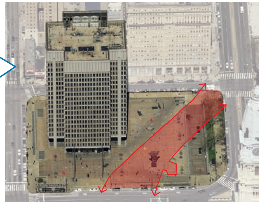
The site presents many obstacles below grade including tunneling for the Broad Street subway and the SEPTA commuter line (in red).
