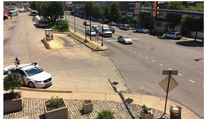
Figure 21: The intersection of Market and 69th Streets experiences a high volume of both pedestrians and vehicles, though the crosswalks are limited to the south and west sides of the intersection. Though there are sidewalks, there are no crosswalks along the bus terminal exit.
