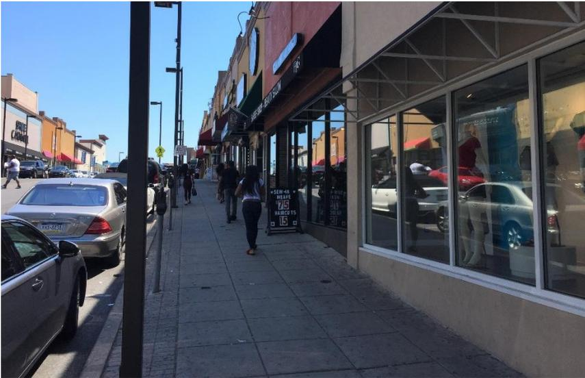
Figure 48: The sidewalk on 69<sup>th</sup> Street includes approximately two feet for both the furnishing zone and frontage zone, leaving about six feet for the pedestrian zone.
