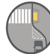
Curb Extension with Daylighting
