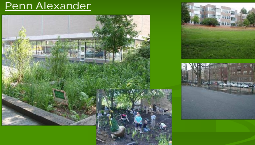
BMPs: Subsurface Infiltration, Rain Garden, Pervious Asphalt
