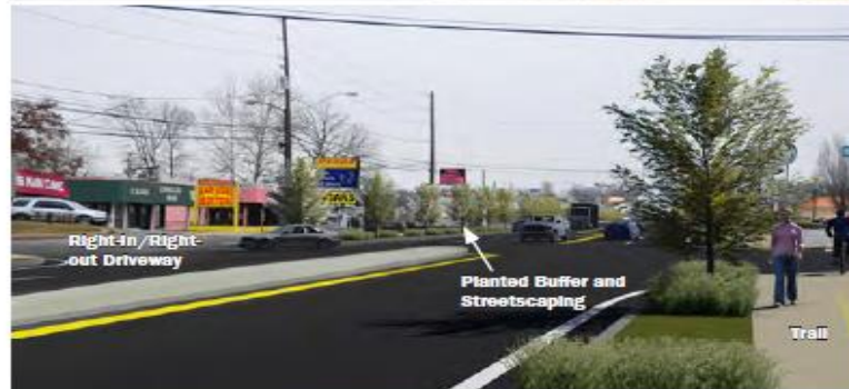
Phase 2: Reconstruction of roadway and installation of multi-use path and streetscaping improvements
